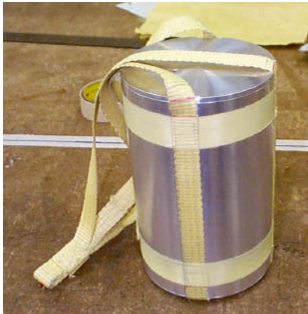
Figure 4. Dummy Telemetry Package Installed in its Bridle (no TM antenna present)
